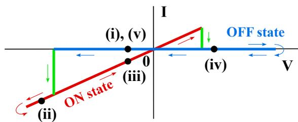
Fig. 2. Schematic diagram of ideal I-V characteristic which shows the memory effect and CAFM measurement points of the procedure from (i) to (v).
