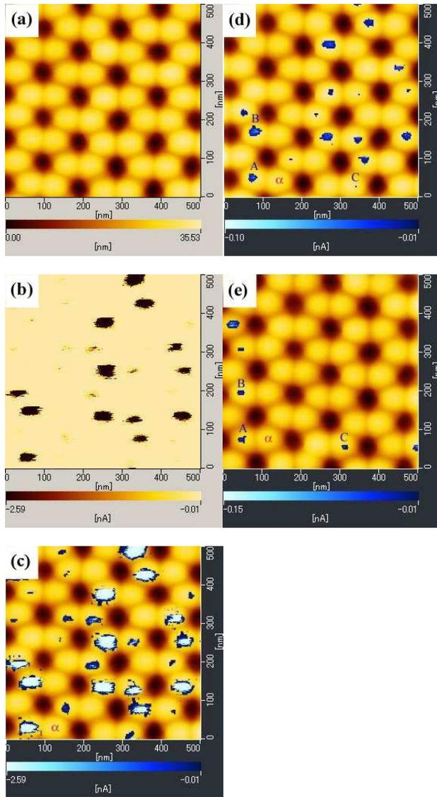
Fig.3. Simultaneously obtained CAFM images (a) surface image, (b)current image, and (c)synthesized image from both (a) and (b) at the first cycle of the procedure (ii), (d) synthesized image at the first cycle of the procedure (iii), (e) synthesized image at the second cycle of the procedure (iii).
