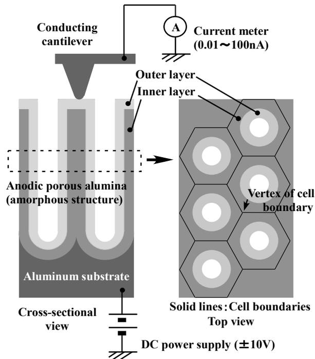
Fig. 1. Schematic diagram of APA film structure.
